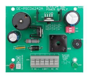
Converts low voltage 16VAC to 28VAC input (typically a plug-in transformer, not included) into 6VDC, 12VDC or 24VDC output. Battery charger output with automatic switchover to DC upon AC failure. Applications include intrusion, access control, video surveillance and other low voltage systems requiring extra power. Includes double-sided foam mounting tape and battery lead wires.
